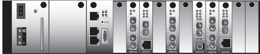
Attached terminal or terminal emulator connected to the DB-9 serial port via a null modem cable .
